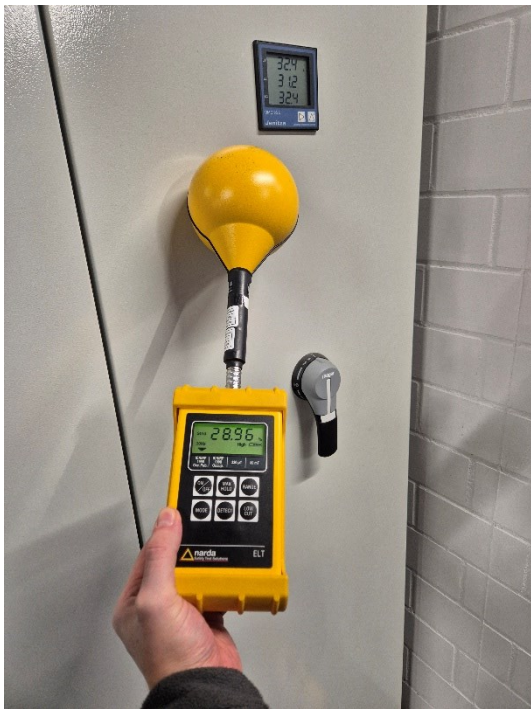
Measurement with Narda ELT-400
